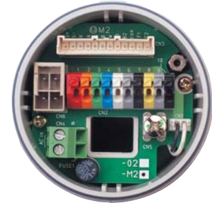
Color Coded Wiring Terminals
