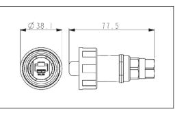
Cable glands optimised for PUR jacket cable to maintain Cat 5e performance Suitable for use with cables from 3.5 to 8mm diameter
