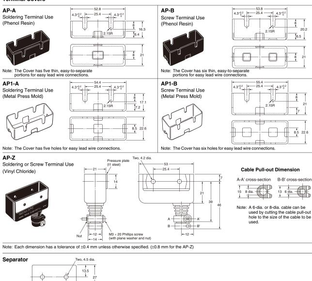
Note: 1. Each dimension has a tolerance of ±0.4 mm unless otherwise specified.
