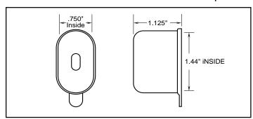
For use on capacitor types MPF/MSF, this neoprene terminal insulator, or 'boot', is used to insulate and protect the terminal area of single section units only. Material is classified 94V-1 when tested per UL94.
