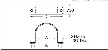
This clamp has a galvanized finish and is designed for use with the round base style motor run capacitor, types MPF.
