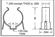
These clips, though designed for capacitors, have varied applications to retain many cylindrical components. They are used extensively in the electrical and electronic industries to hold spindles, condensers, capacitors, tubes, rods and conduit. Clips have phosphate and oil finish.
