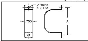
This clamp has a galvanized finish and is designed for use with the flat oval base style AC capacitors, types MPF/MSF.
