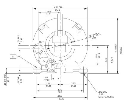
1 DRAWING NOT TO SCALE, CONTACT FACTORY FOR SCALE CAD DRAWING. 2 CONTACT FACTORY FOR BLOWER MODEL LENGTHS NOT SHOWN.
