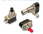
The P26-Series pushbutton switches are single pole, AC rated for 8 amps at 125 VAC and suitable for shallow back Electrical Life panel applications. These switches are momentary action with a medium actuation force (13 oz. typical). The P26-Series switch is equipped with a slow-make, slow-break 100,000 cycles contact mechanism. Typical applications include usage for an Alarm or Warning Device, as well as Test and Measurement Equipment.
