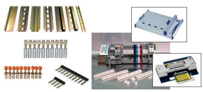
Last, but not least, the indispensable extras. End Stops prevent terminal blocks and other components from sliding laterally on the rail. End Plates close off the last terminal in a row of terminals. Isolation Partitions provide visual separation of terminal groups and ensure electrical isolation between adjacent terminals of different potentials. A wide selection of insulated and uninsulated ferrules is offered for your applications and whenever stranded flexible wires must be terminated.
