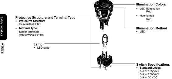
Note: A165E Emergency Stop Switch must be ordered as a set. No LED is installed for the non-lighted models.
