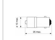
Part Number: 1860613W3D Serial Number: 18606 Based LED type: StarLED Size (inch): T-3 1/4 Size (mm): T10 Housing Size: 10x25mm
