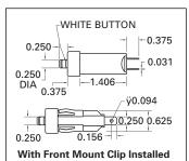
PANEL MTG. HOLE FOR PANEL THICKNESS 1/32 THRU 1/8 Panel Mounting Hole
