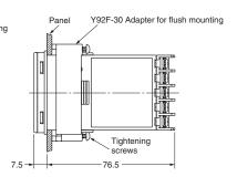
Note: 1. The recommended panel thickness is 1 to 4 mm.
