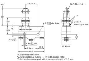
OF max. 540 gf 114 gf RF min. 1.8 mm PT max OT min. 3.58 mm MD max. 0.06 mm OP 33.4±1.2 mm
