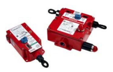
CPS Series Cable Pull Safety Switches provide a readily accessible emergency stop signal. This is a cost-effective means compared to using multiple emergency stop push-buttons. (Cable Pull Safety Switches are not, however, to be used as a means of personnel safeguarding. They may be used to prevent further injury or damage to equipment when used for emergency stop signaling.)
