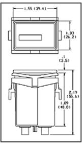
$^{\star}$  Panel cutout dimensions are  $\pm$  .010 tolerance All dimensions shown in inches and (metric)
