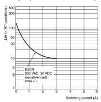
Note: Do not connect a DC load to a Controller with a Long-life Relay
