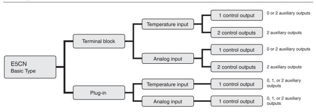
Note: Models with one control output and one or two auxiliary outputs and models with two control outputs can be used for heating/cooling control.
