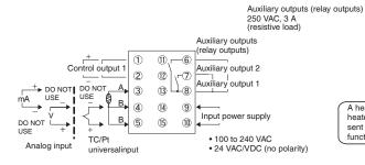
A heater burnout alarm, heater short alarm heater overcurrent alarm, or input alarm is sent to the output to which the alarm 1 function is assigned.
