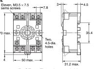
Terminal Layout/Internal Connections (Top View)
