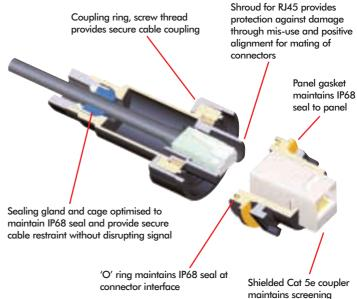
Over moulded assembly provides IP68 cable seal
