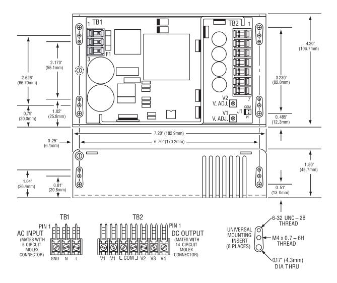
INPUT & OUTPUT CONNECTIONS: 6-32 SCREW WIRE CLAMPS ON 0.312" (7.9mm) CENTERS, 0.045" (1.1mm)
