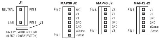
J1/J2 MATES WITH MOLEX (SERIES 2139 or SERIES 41695) .156" (4mm) CENTER CRIMP TERMINAL HOUSING OR EQUIVALENT
