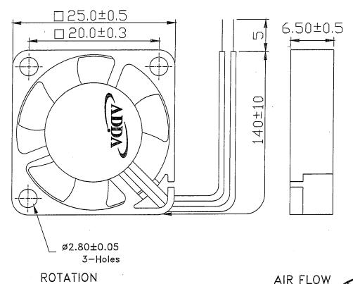
LEAD WIRES: UL 1571, AWG28, L = 140 +/- 10 mm Red = positive; Black = negative.
