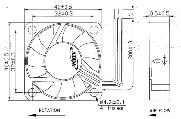
LEAD WIRES: UL 1007, AWG26, L = 300 +/- 10 MM Red = positive; Black = negative.
