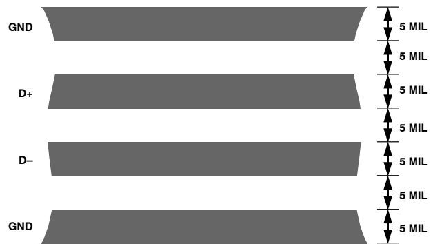
Figure 23. Typical Arrangement of Signal Tracks
