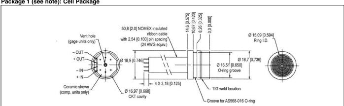
Note: Non-concentricity effects at the diaphragm weld area may cause runout of up to ±0.006 in between the upper and lower portions of the sensor body. (It is recommended to use a counter bore to mate with this device to allow for this non-concentricity).
