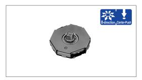
Typical Specifications Items **Specifications Swich ON position** 7° max. **Operating force** 0.8±0.5N **Push operating force**  $2.5 \pm 1.5N$ Travel (Push operation) 0.3±0.2mm **Push strength** 30N Rating (max.) (Resistive load) 10mA 5V DC **Operating life** Each direction 500,000cycles Insulation resistance  $50M\,\Omega$  min. 50V DC Voltage proof 50V AC for 1minute
