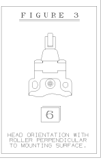
HEAD ORIENTATION WITH ROLLER PERPENDICULAR TO MOUNTING SURFACE.
