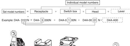
\* The D4A-□N without the above accessories is not compatible with the D4A-□.
