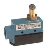
Enclosed Switches Series E6: Top Roller Plunger Actuator; 1NC 1NO SPDT Snap Action; 0.5 in - 14NPT conduit
