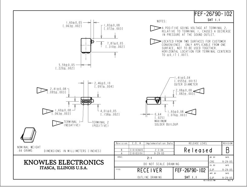
THE FEF-26790-i02 IS A FERROFLUID DAMPED EF RECEIVER.
