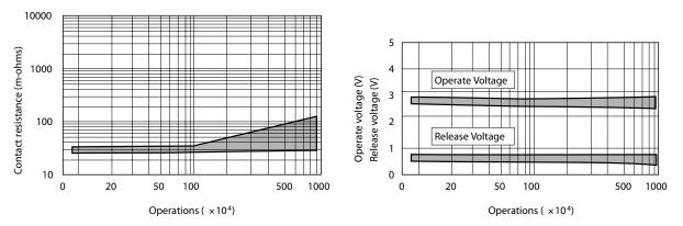
RUNNING TEST (Load) (Load: 50 V.DC 0.1 A resistive, Driving: 5V.DC, 5 Hz, 50% duty, Ambient temperature: 85 degree C, Sample: MR82-5USR 10 pieces)
