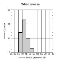
5-(2). Operation noise distribution LK-F (Height: 10 mm, Standard) Measuring conditions Sample: LKF1aM-12V-1-5, 50pcs Background noise: approx. 20dB Coil voltage: 12V DC Equipment setting: "A" weighted Single part (refer to figure below) With diode
