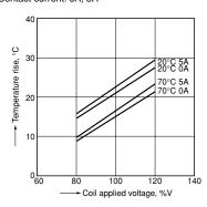
2-(2). Coil temperature rise (TV-8 type) Sample: LKF1aMQ-12V-1-8, 6 pcs. Point measured: coil inside Contact current: 0A, 8A
