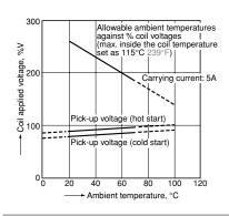
3-(2). Ambient temperature characteristics and coil applied voltage (TV-8 type)
