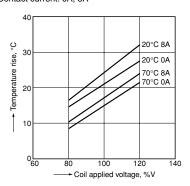
3-(1). Ambient temperature characteristics and coil applied voltage (TV-5 type)
