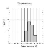
5-(3). Operation noise distribution LK-S (Height: 25 mm) Refer to comparison Measuring conditions Sample: LKS1aF-12V, 50pcs Background noise: approx. 20dB Coil voltage: 12V DC Equipment setting: "A" weighted Single part (refer to figure below) With diode
