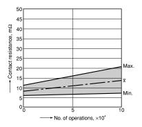
4-(2). Electrical life test (8A 277V AC, resistive load) Sample: LKF1aMQ-12V-1-8, 6 pcs. Operation frequency: 20 times/min. (ON/OFF = 1.5s: 1.5s) Ambient temperature: 20°C 68°F
