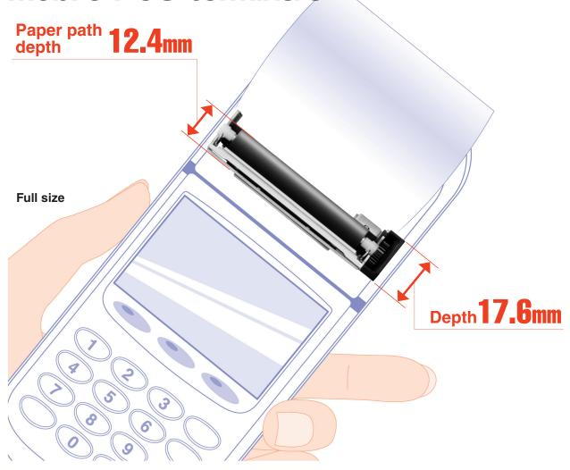
Compact mechanism pursuing smaller size and less weight, contributes to flexibility of set design.
