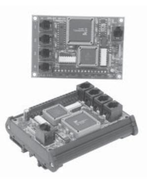
If your application requires a single axis to operate in "host mode", you can connect any of our programmable  $Si^{TM}$  drives directly to your PC via the SiNet Hub 444 and invoke the  $Si^{TM}$  Command Language (SCL).
