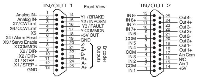
Note - this connector is standard on S version and only on S and Q versions with expanded I/O.
