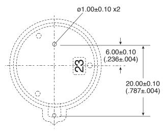
Recommended PCB Layout Component Side
