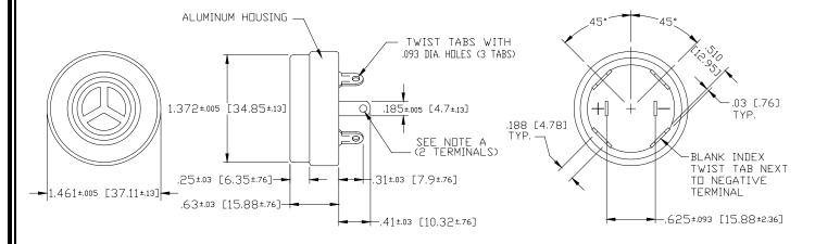
NOTE A: TERMINALS - .032 STEEL, TIN PLATED WITH .093 DIA. WIRE HOLE, WILL ACCEPT STANDARD 3/16 QUICK CONNECT
