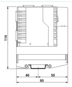
The illustration shows the head station FL SWITCH MM HS with interface module
