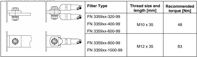
The recommended torque is based on a strength class of 8.8 (ISO 898-1). Any other screw type or material needs to be checked by the installer.
