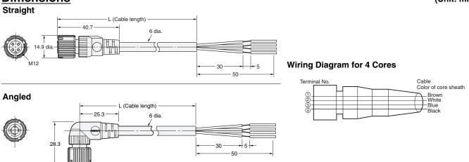
Note: The overmolding on the Standard Cable (XS5F-D42 -- 80-A) and the Oil-resistant Polyurethane Cable (XS5F-D42 -- 80-P) is black, and the overmolding on the Vibration-proof Robot Cable (XS5F-D42□-□80-F) is gray.
