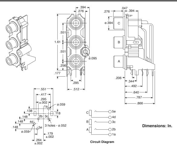
PCB Hole Layout (Bottom View)
