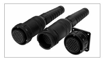
Amphenol's MP-41 series of multipin connectors utilise the same design principals of the rugged Mil-C-5015 military connectors. They can withstand high shock and vibration environments and are ideal for tough on-road applications. Featuring a quick mating bayonet coupling with an audible full mating feature ensures a positive connection every time. Available from 13 to 150 pins with gold plated "combo"\* contacts supplied with each connector as standard.
