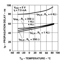
Figure 7. Typical propagation delay vs. temperature.
