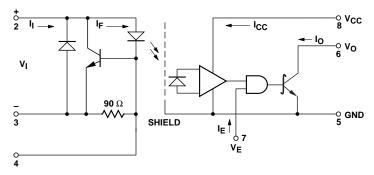
USE OF A 0.1  $\mu F$  BYPASS CAPACITOR CONNECTED BETWEEN PINS 5 AND 8 IS REQUIRED (SEE NOTE 1).
