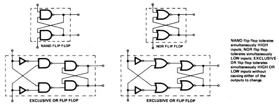
Figure d. Flip-flop configurations.
