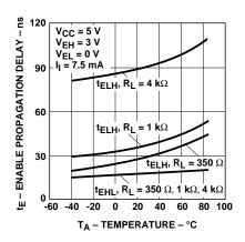
Figure 11. Typical enable propagation delay vs. temperature.
