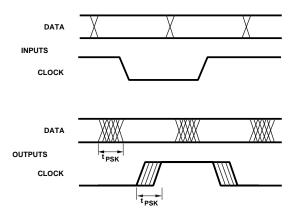
Figure 17. Parallel data transmission example.
