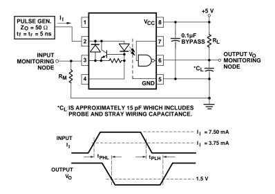
Figure 6. Test circuit for  $t_{\mbox{\tiny PHL}}$  and  $t_{\mbox{\tiny PLH}}.$
