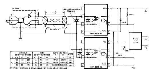
Figure c. Polarity reversing, split phase.
