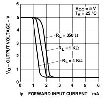
Figure 4. Typical output voltage vs. forward input current.
