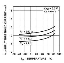
Figure 14. Typical input threshold current vs. temperature.
