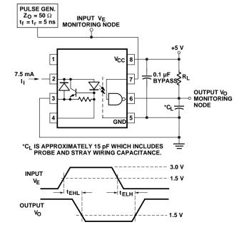
Figure 10. Test circuit for  $\mathbf{t}_{\text{\tiny EHL}}$  and  $\mathbf{t}_{\text{\tiny ELH}}.$
