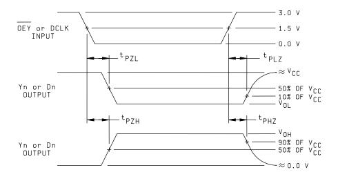
FIGURE 4. Switching waveforms and test circuit.
