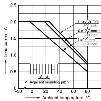
4.-(2) Characteristics of load current vs. ambient temperature for adjacent mounting
