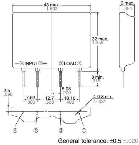
**Mounting hole location (Bottom view)**
