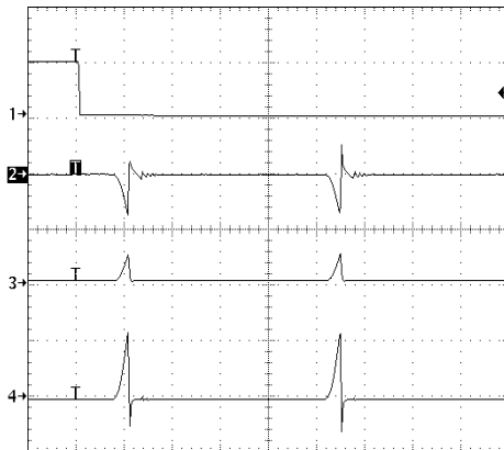
FIGURE 12. FAULT to Short Response ( t_{\text{cyc}} )
