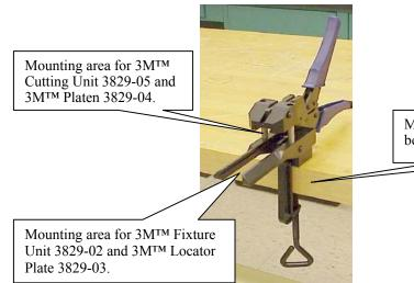
Mount the  $3M^{TM}$  Hand Press to a bench using the  $3M^{TM}$  Bench Clamp.
