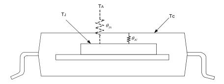
Notes: 2.  $\theta_{JA}$  should be confirmed with heat sink thermal resistance. If there is no heat sink contact,  $\theta_{JA}$  will almost be the same as  $\theta_{JC}$ .
