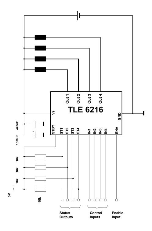
The blocking capacitor C is recommended to avoid critical negative voltage spikes on VS in case of battery interruption during OFF-commutation.
