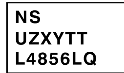
Top View NS - Std NS Logo U - Wafer Fab Code Z - Assembly Plant Code XY - 2 Digit Date Code TT - Die Run Traceability L4856LQ - LM4856LQ
