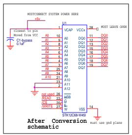
On the next page, pin by pin comparisons of the two show all pins are the same except for the bypass capacitor moving to pin 1 and connected to system power, +5v. Pin 28 must now be unpowered and open.
