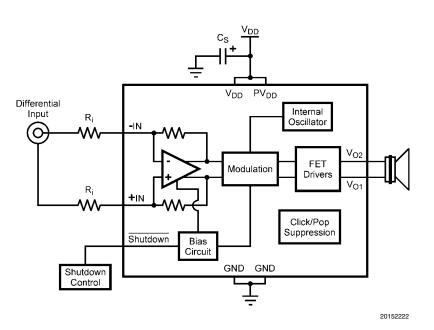
FIGURE 2. Differential Input Configuration
