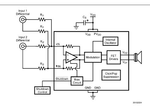
FIGURE 4. Dual Differential Input Configuration
