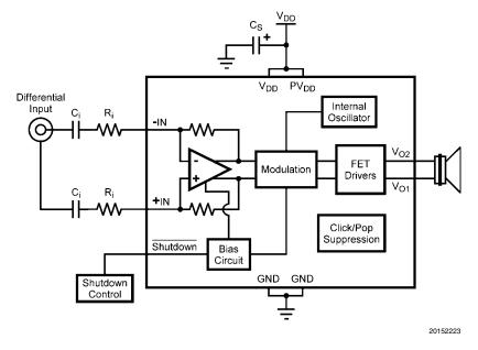
FIGURE 3. Differential Input Configuration with Input Capacitors
