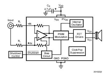
FIGURE 1. Typical Audio Amplifier Application Circuit
