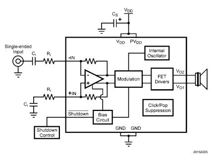
FIGURE 5. Single-Ended Input Configuration
