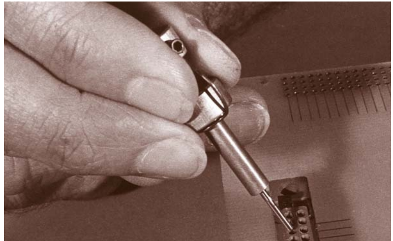
INSERT EXTRACTION TOOL WITH PLUNGER RETRACTED
